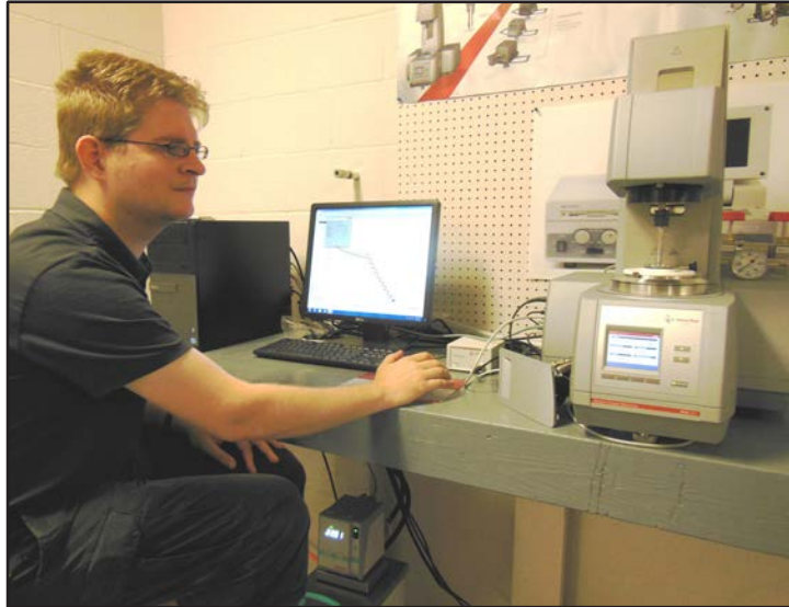
Figure 1. Dr. Dimitri Feys Testing Cement Paste using Anton-Paar MCR 302 Rheometer
